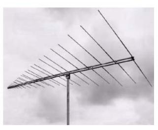
The Model LP-1018BA log periodic dipole antenna has been designed for transmission or reception in either oriented position – providing a vertical or horizontal polarization. Applications for this antenna include point to point, ground to air, surveillance, etc. The broadband width of 30 through 1100 MHz, together with its high gain of 8.0 dB, and high front to back ratio of 15 dB, yield an antenna of infinite possibilities and applications.
